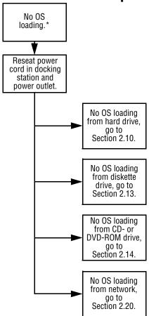
\*NOTE: Before beginning troubleshooting, always check cable connections, cable ends, and drives for bent or damaged pins.
